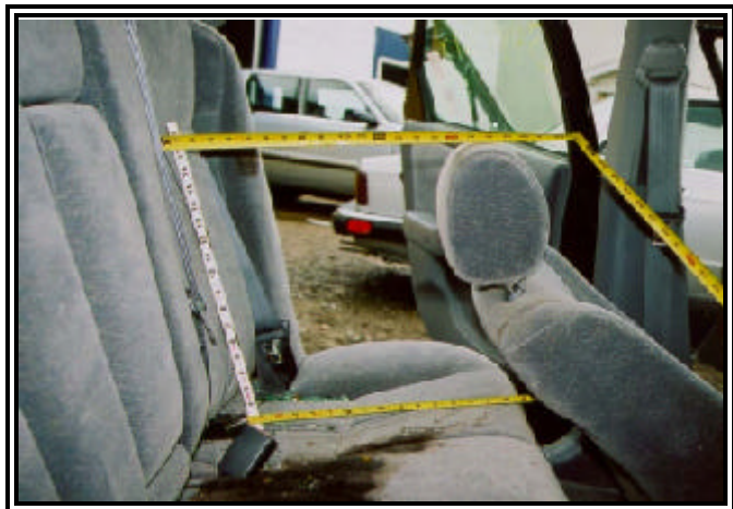
Figure 13: Measurements of the residual left rear interior space.
