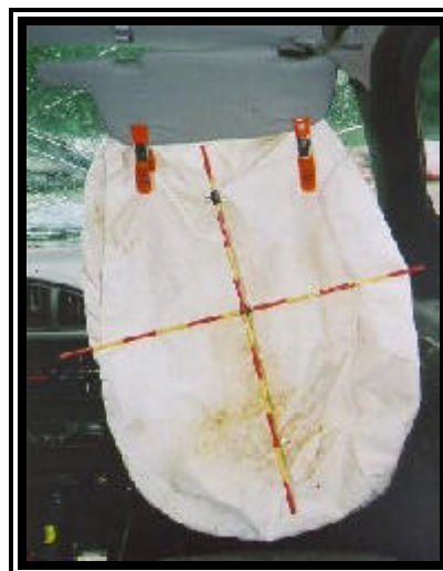
Figure 8. 1996 Geo Metro LSI deployed passenger air bag.
