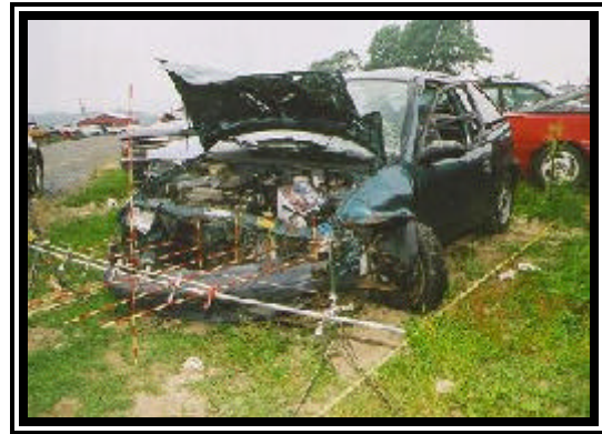
Figure 3. Front left damage to the 1996 Geo Metro LSI.
