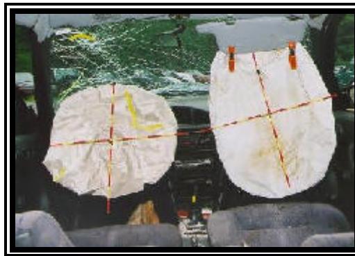
Figure 6. 1996 Geo Metro LSI deployed frontal air bag system.
