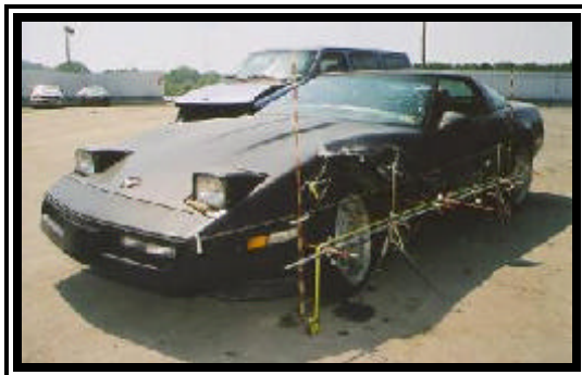
Figure 4. Left front side surface damage to the 1990 Chevrolet Corvette.
