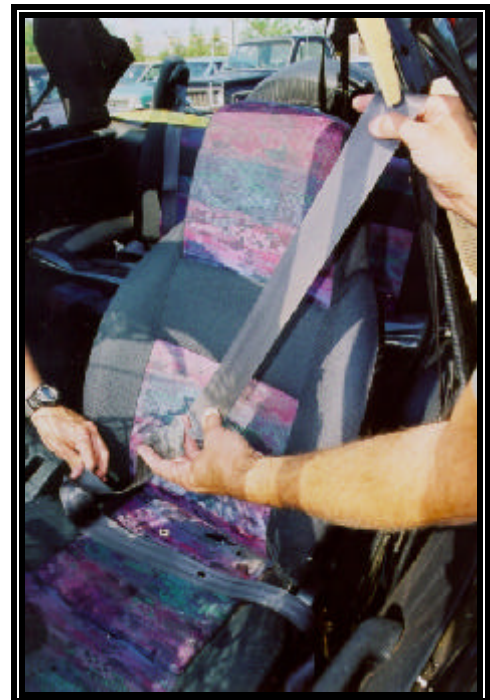
Figure 9: Reconstructed belt path for the Geo's driver.
