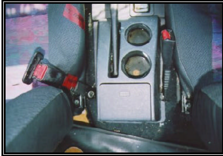
Figure 13: Overhead view of the inboard buckles.
