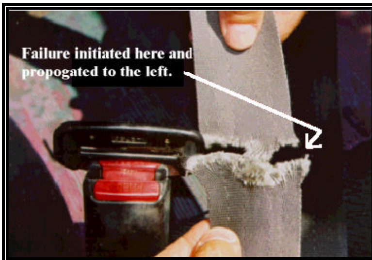
Figure 12: View of the latch plate and webbing separation.
