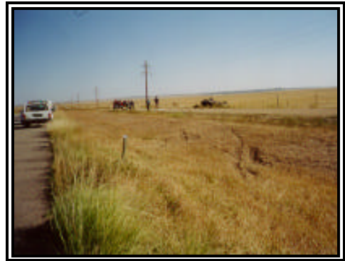
Figure 4. Gouges in the grassy ditch and damaged delineator post
