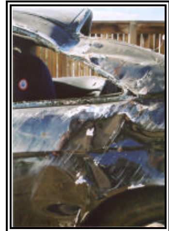
Figure 8. Damage from the first delineator post
