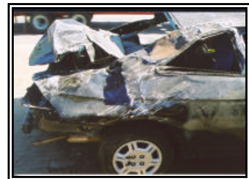
Figure 9. Abraded right rear quarter panel and displaced trunk lid
