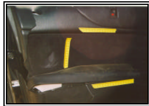
Figure 10. Damaged left front door interior panel
