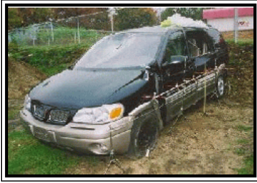
Figure 4. Windshield and left side surface damage to the 2000 Pontiac Montana.
