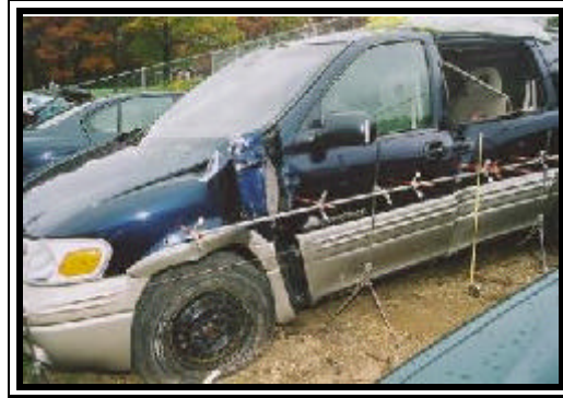
Figure 5. Left side view with direct contact damage to the A-pillar and B-pillar.
