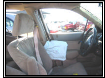
Figure 10. Deployed driver's side impact air bag
