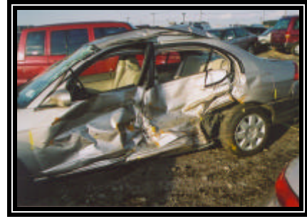
Figure 4. Left side damage to the Honda Civic
