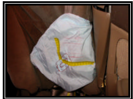
Figure 11. View showing red linear transfers on the outboard aspect of the driver's side impact air bag
