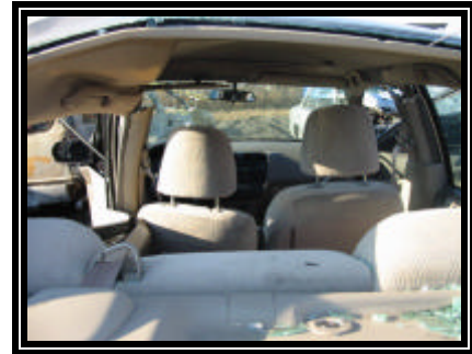
Figure 7. View through the backlight showing lateral intrusion
