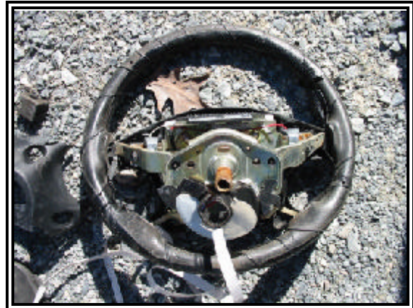
Figure 11: Fractured steering shaft.
