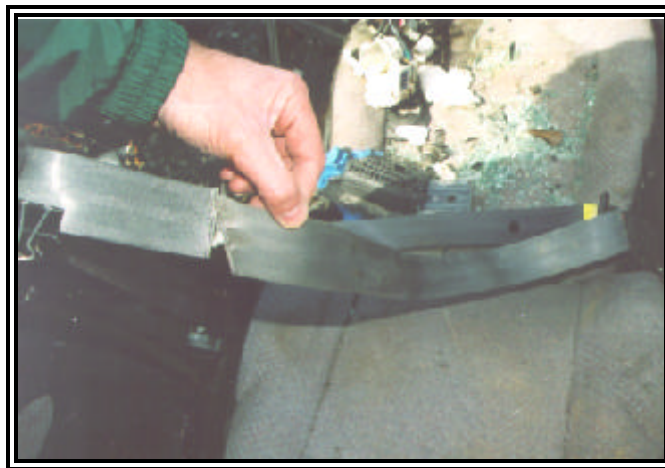
Figure 13: View of the cut driver seat belt webbing.
