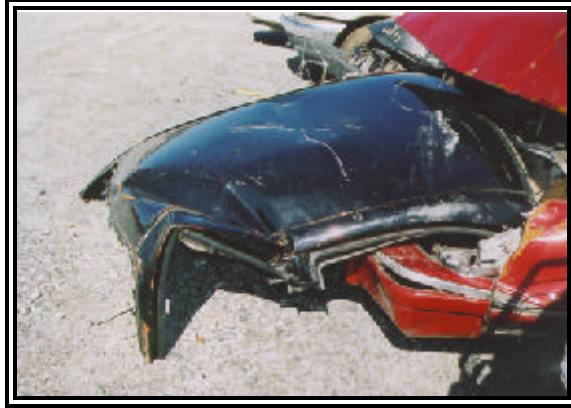
Figure 7: View of roof and left A-pillar damage.
