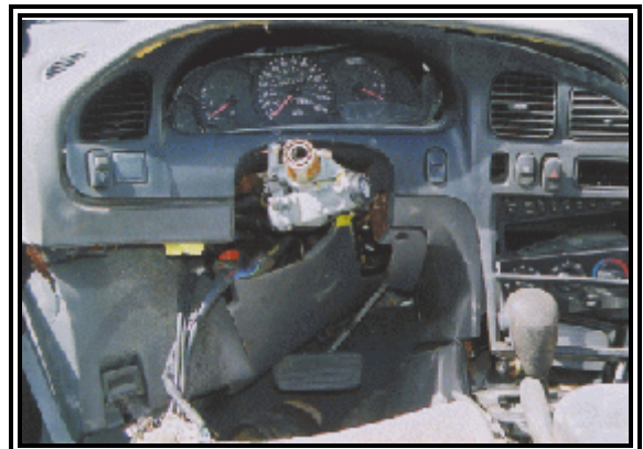
Figure 9: Knee bolster deformation.
