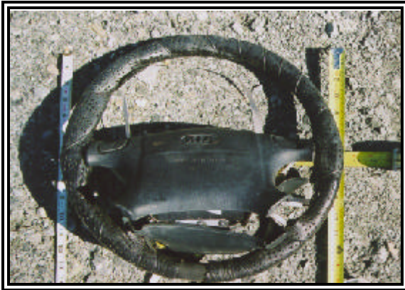
Figure 10: View of the steering wheel rim deformation and non-deployed driver air bag.
