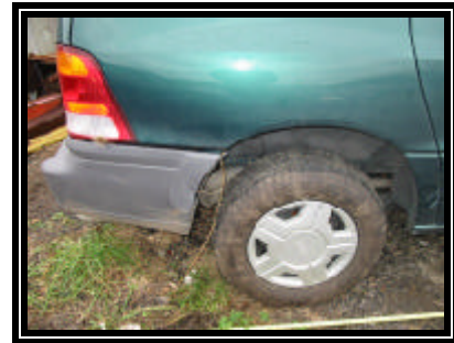
Figure 5. Right rear damage from the sideswipe impact
