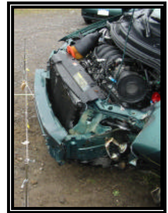
Figure 8. Lateral view of direct and induced frontal damage
