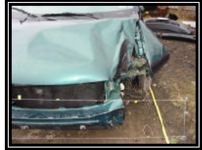
Figure 7. Direct damage from pole impact
