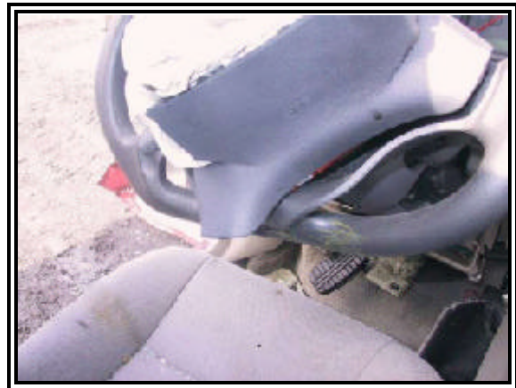
Figure 6: Deformed steering wheel rim.
