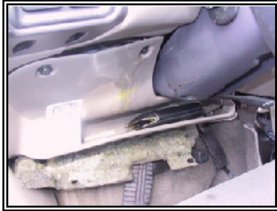
Figure 7: Lower extremity contacts to the intruding bolster.
