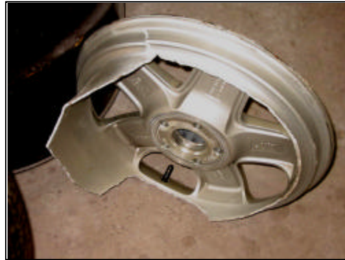
Figure 7. View of outboard aspect of the fractured alloy wheel
