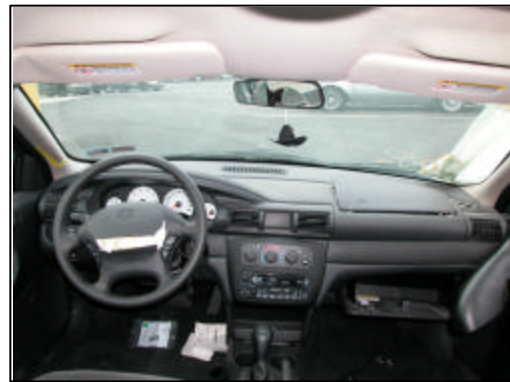
Figure 8. View of instrument panel area and fractured rear-view mirror
