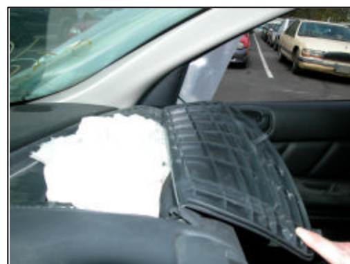
Figure 12. Lateral view from left-to-right showing excursion of front right passenger's air bag cover flap
