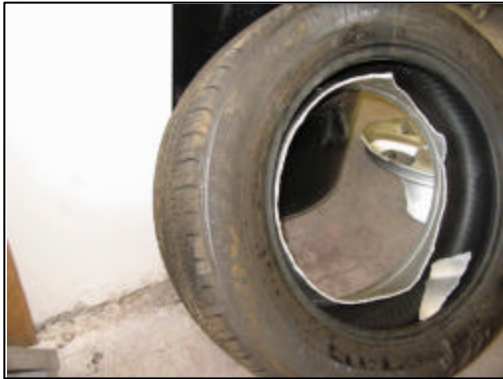
Figure 6. View of front right wheel and inboard aspect of fractured alloy wheel
