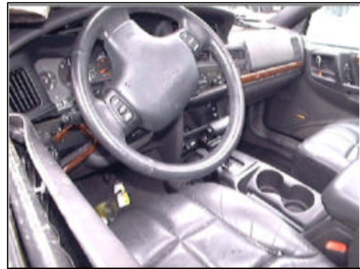
Figure 7. Interior view showing occupant contact damage
