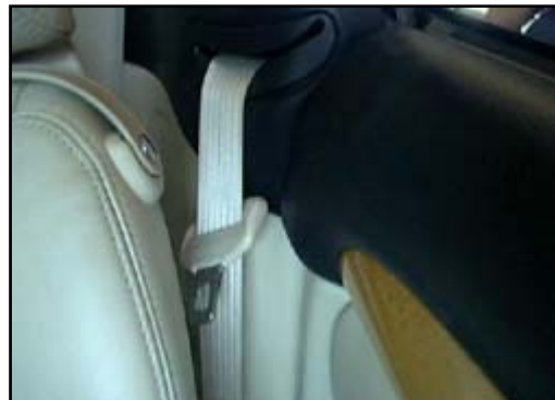
Figure 8. Fired front left safety belt pretensioner.
