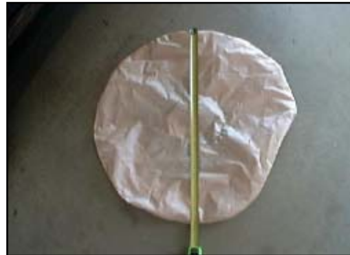
Figure 9. Driver’s air bag cut out of module.
