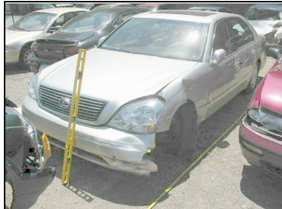
Figure 3: Overlapping damage from embankment and pole impacts at front left corner
