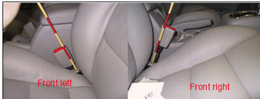
Figure 12. Driver's pretensioner fired, front right passenger pretensioner did not fire
