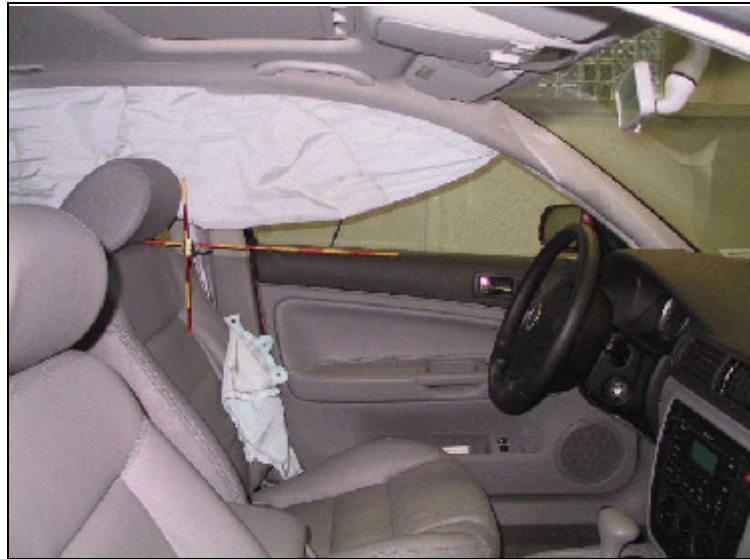
Figure 10. Driver's seat back mounted side impact air bag and side air curtain.
