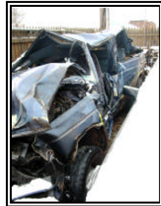
Figure 10. Left side damage from pole impact
