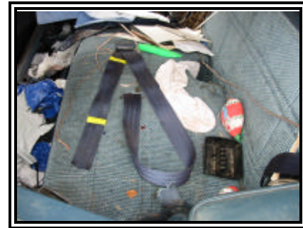
Figure 13. Cut rear left manual restraint
