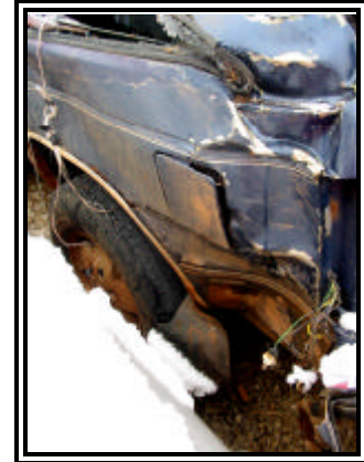
Figure 7. Initial contact damage
