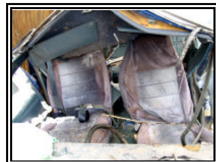
Figure 11. View through windshield showing intrusions
