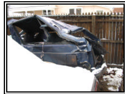
Figure 9. Damage to rear aspect of roof and left C-pillar
