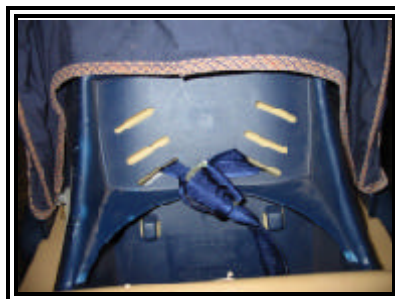
Figure 17. View of harness straps through the adjustment slide
