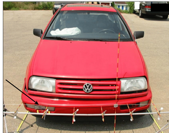
Figure 9: Case vehicle's frontal damage with contour gauge present at bumper level; Note: arrow indicates impact location of pickup's trailer hitch (case photo #15)
