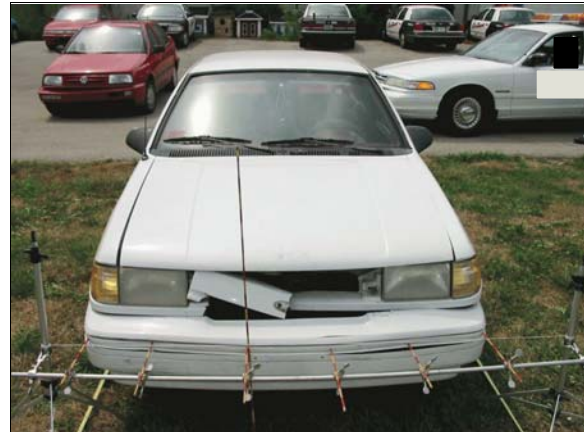
Figure 3: Ford Tempo's frontal damage from impact (1 st event) to back of case vehicle; Note: contour gauge present a bumper level (case photo #67)
