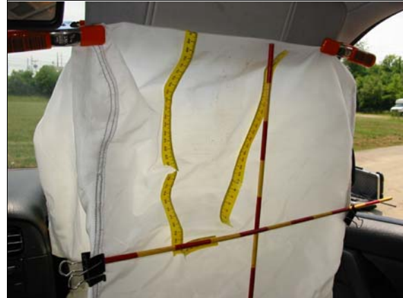
Figure 12: Case vehicle's deployed front right passenger air bag showing skin smudges in upper left quadrant of bag's front surface (case photo #53)
