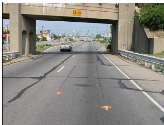
Figure 1: Southward travel path of Ford pickup, case vehicle, and Ford Tempo in outside lane of southbound roadway, showing Tempo’s straight line, pre-crash skid marks (case photo #01)
