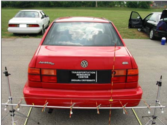
Figure 2: Damage to case vehicle's back bumper from impact (1 st event) by Tempo; Note: contour gauge present at bumper level (case photo #23)
