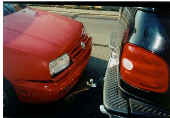
Figure 4: On-scene view of final rest positions of case vehicle and Ford pickup (2 nd event), showing rear-end impact configuration; Note: trailer hitch on pickup's back bumper damaged case vehicle's front (case photo #12)
