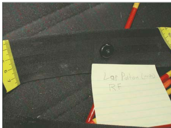
Figure 14: Close-up of case vehicle's front right seat belt webbing showing wear marks and body fluids (case photo #44)
