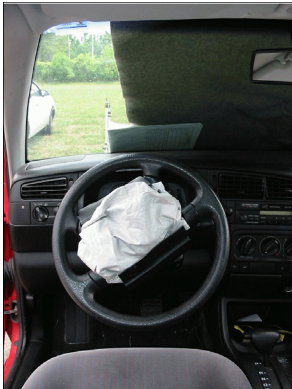
Figure 6: Vertical view of case vehicle’s driver seating area showing deployed driver air bag and no apparent occupant contact evidence on steering wheel rim or greenhouse areas (case photo #36)
