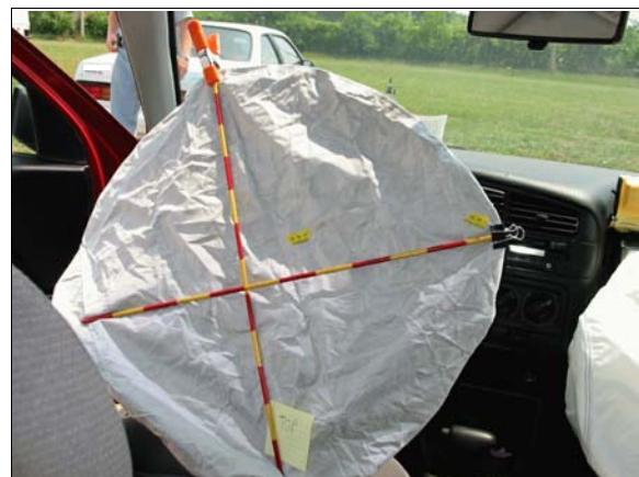
Figure 11: Case vehicle's deployed driver air bag showing faint smudges (i.e., yellow tape); Note: steering wheel has been rotated approximately 170 degrees clockwise (case photo #46)
