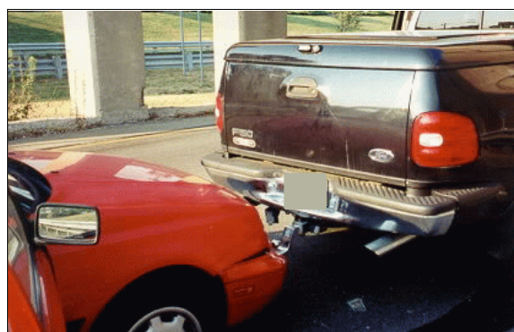
Figure 18: On-scene view of back of Ford pickup showing no obvious damage to back bumper but damage to trailer hitch (case photo #11a)
