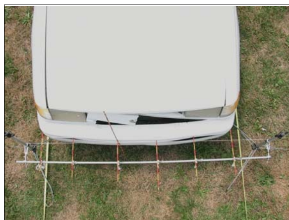
Figure 17: Overhead view of Ford Tempo's frontal damage from impact with case vehicle (1 st event) with contour gauge positioned at bumper level (case photo #70)
