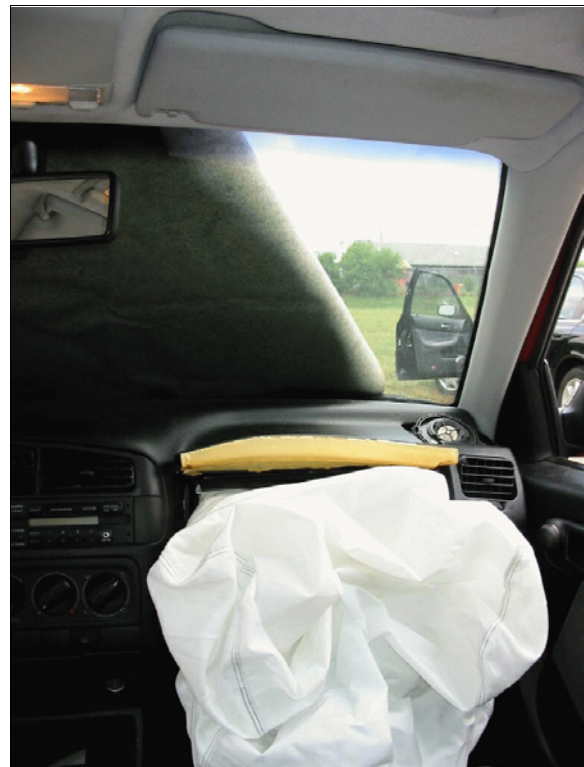
Figure 7: Vertical view of case vehicle’s front right passenger seating area showing deployed front right passenger air bag and underneath surface of air bag module’s cover flap; Note: no contact evidence on windshield’s glazing or on right “A”-pillar, sun visor, or roof (case photo #65)
