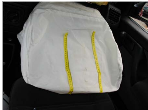
Figure 13: Top surface of case vehicle's deployed front right air bag; Note: blood and scuff marks (case photo #60)
