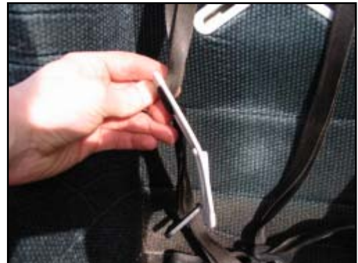
Figure 12. Horizontal view of the deformed harness retainer clip
