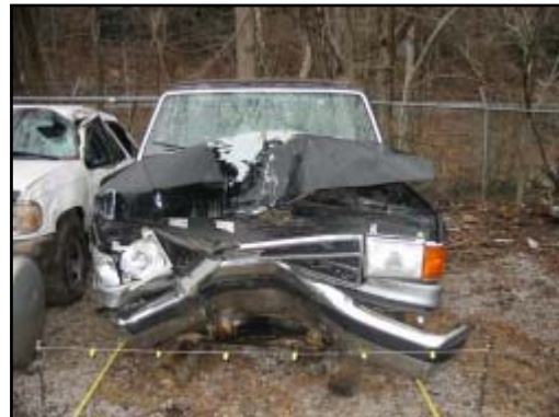
Figure 1. Damaged Ford F-150 pickup truck
