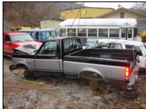
Figure 6. Left side view showing displacement of the cargo box
