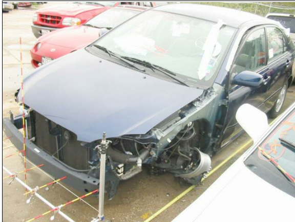
Figure 6: Elevated view of case vehicle's very narrow front left corner impact; Note: left fender and left front wheel were torn off during impact (case photo #17)
