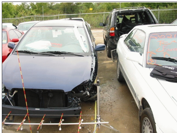
Figure 4: Case vehicle's very narrow front left corner impact viewed along left side (case photo #16)
