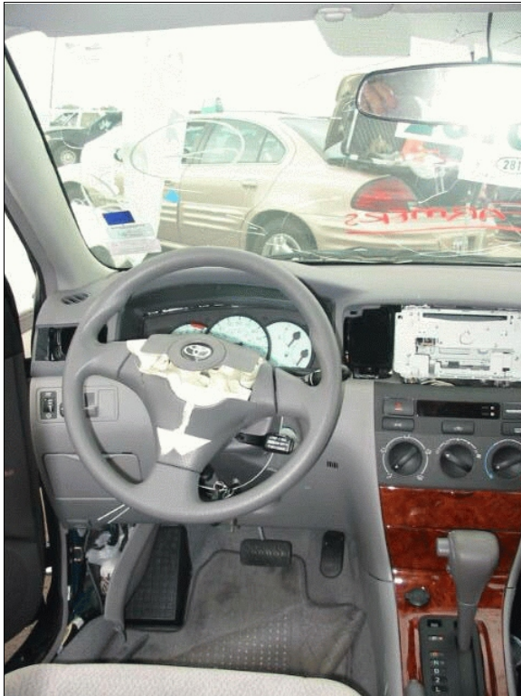
Figure 10: Vertical view of case vehicle's driver seating area showing residual of deployed driver air bag absence of obvious occupant contact evidence (case photo #33)
