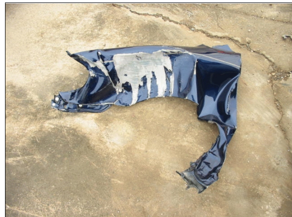
Figure 9: Case vehicle's left fender torn-off during impact with light pole; Note: slot for left headlight is towards left of photo (case photo #18)
