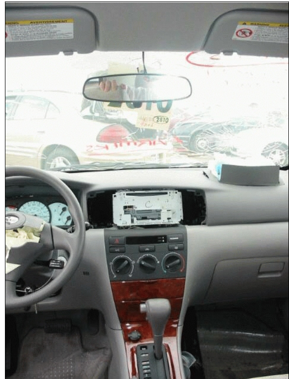
Figure 11: Vertical view of case vehicle's front seating and greenhouse areas showing absence of obvious occupant contact evidence and cracked right windshield's glazing—cracked from contact by front right air bag's fabric (case photo #34)
