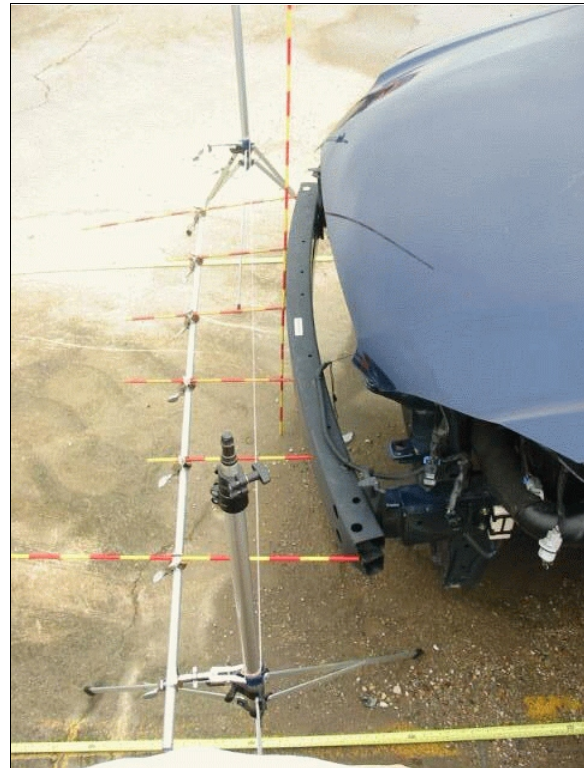
Figure 7: Case vehicle's very narrow front left corner impact viewed along front reference line (case photo #12)
