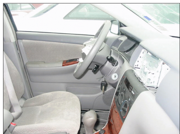
Figure 12: Case vehicle's undeformed steering wheel viewed from right and left "A"-pillar and side interior surfaces without occupant contact evidence (case photo #37)
