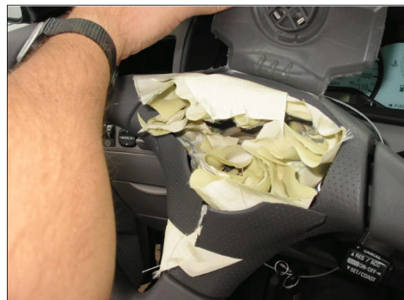
Figure 14: Interior of case vehicle's driver air bag module showing residual of cutout air bag (case photo #42)
