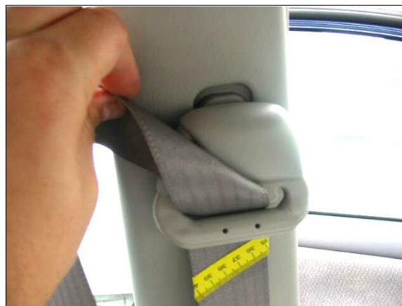
Figure 16: Case vehicle's driver "D"-ring and webbing showing trace evidence of usage on webbing (case photo #29)
