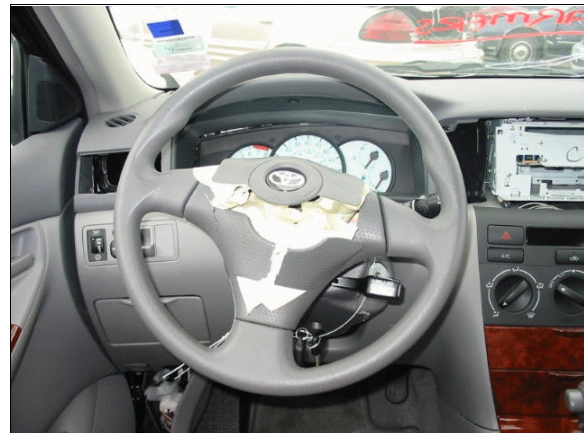
Figure 13: Case vehicle's steering wheel showing deployed driver air bag module's cover flaps and residual of cutout air bag's fabric (case photo #39)
