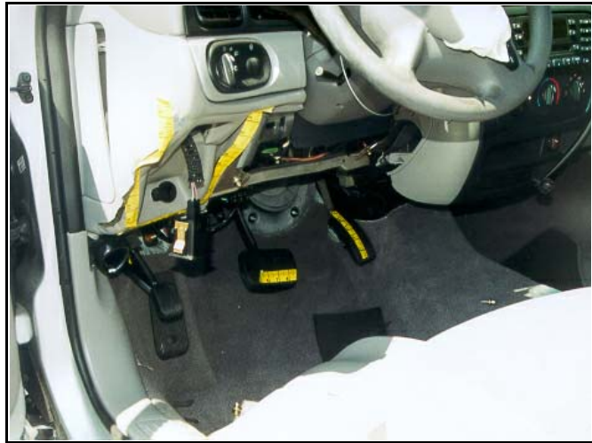
Figure 3. Damage to instrument panel.
