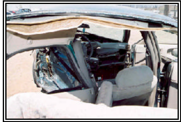
Figure 10: Rear view depicting the intrusion.
