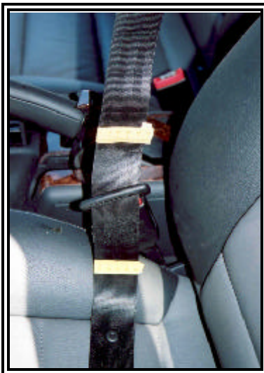
Figure 7: Webbing abrasion at the latch plate.
