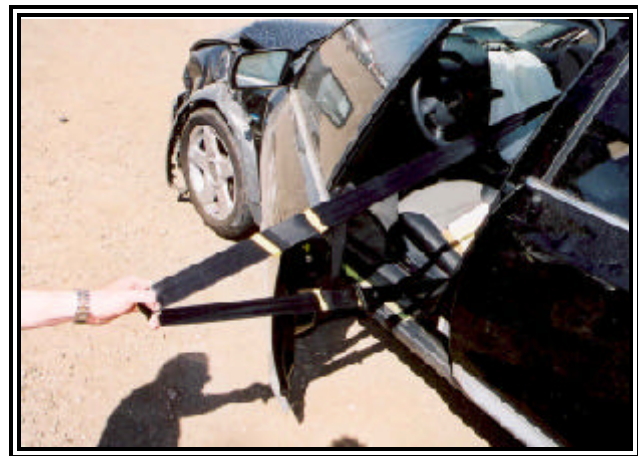
Figure 8: View of the webbing abrasions.
