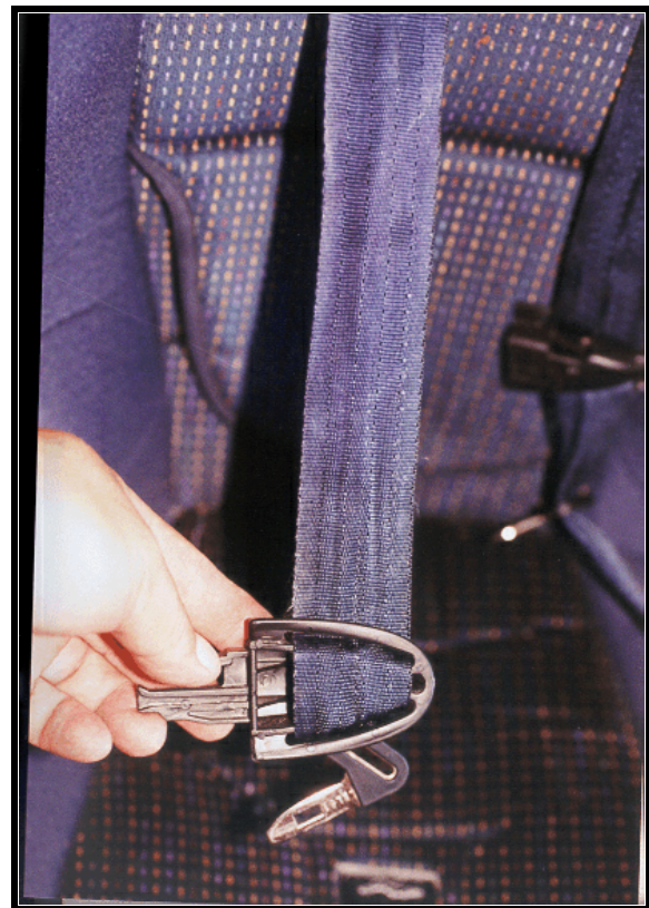
Figure 11. Loading marks to child safety seat harness
