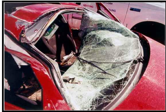
Figure 8. Windshield integrity loss
