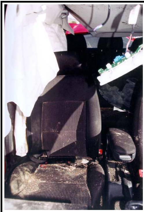
Figure 13. Front right-side air bag and head impact air bag activated
