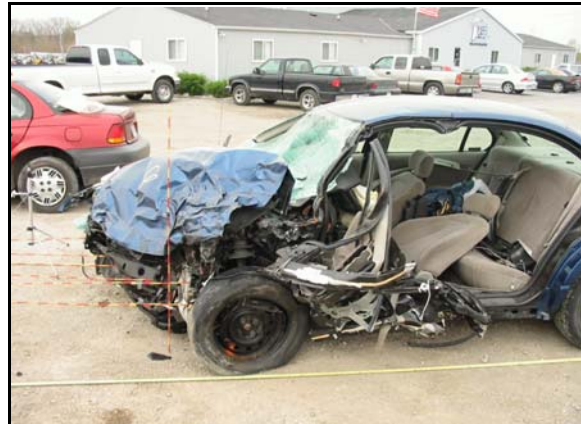
Figure 5: Case vehicle's left side, showing driver's seat area (doors removed for extrication) (case photo #20)
