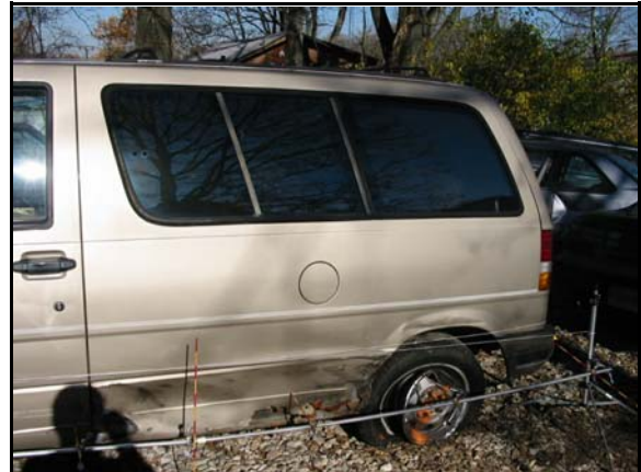
Figure 7: Left side of Ford Aerostar, showing area of maximum crush (case photo #57)
