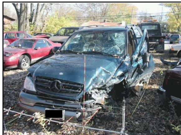
Figure 8: Front and left side of Mercedes SUV, showing heavy damage from offset frontal impact (case photo #70)
