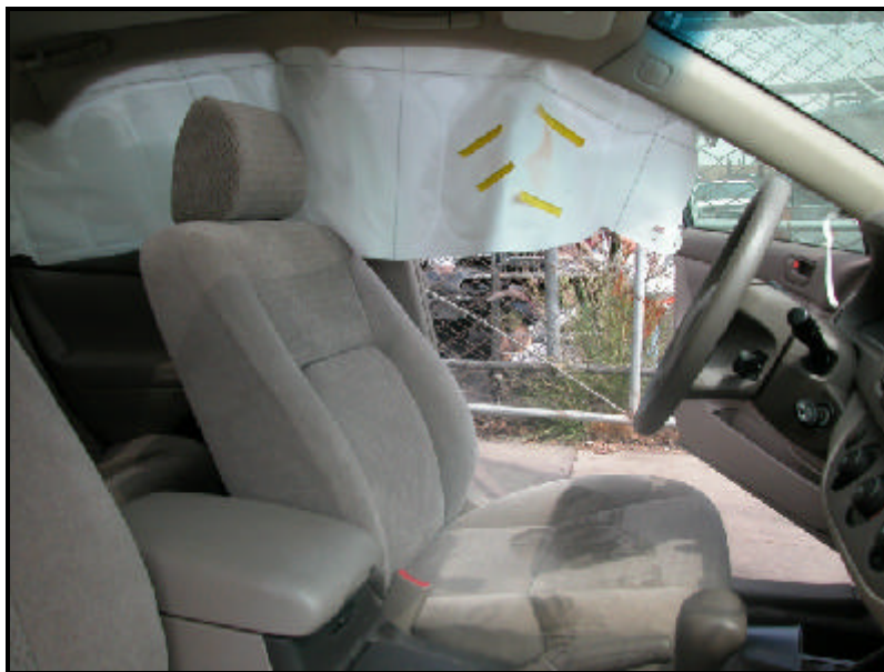
Figure 12. Driver's seat-contact to side air curtain
