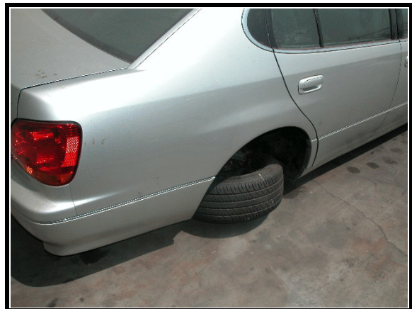
Figure 5. Right rear tire damage from curb impact
