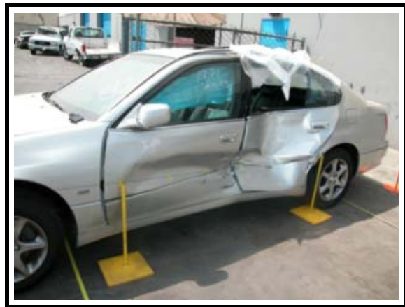
Figure 3. Case vehicle left side damage.
