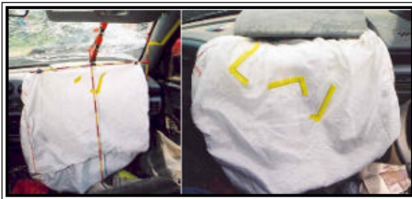
Figure 8. Contact evidence to the 1995 Chevrolet Lumina deployed front right passenger air bag.
