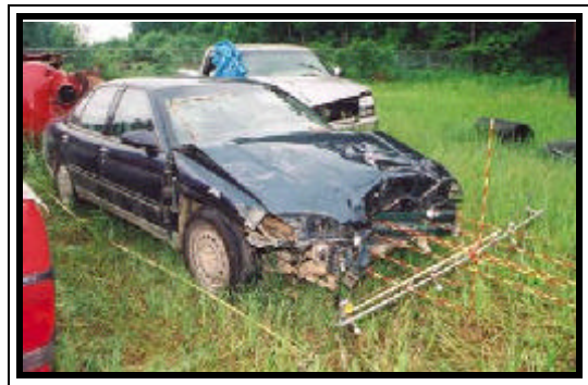
Figure 4. Frontal damage to the 1995 Chevrolet Lumina.
