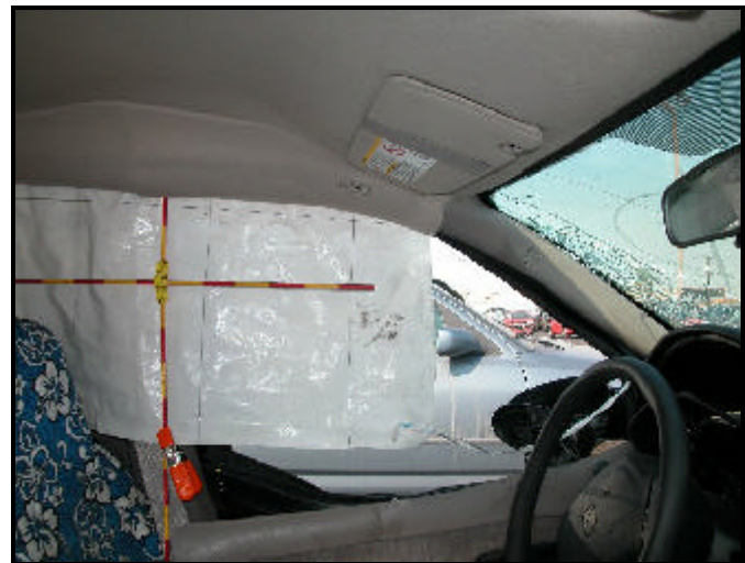
Figure 10. Interior view, head curtain side air bag
