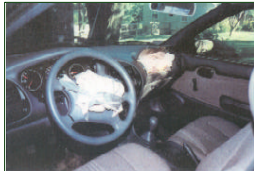
Figure 7. Deployed frontal air bag system in the Geo Prizm.
