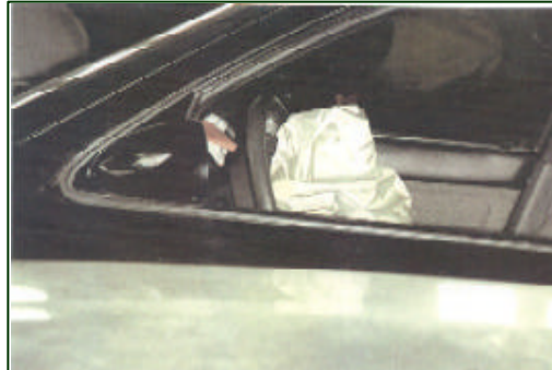
Figure 9. Lateral view of the deployed front left air bag.
