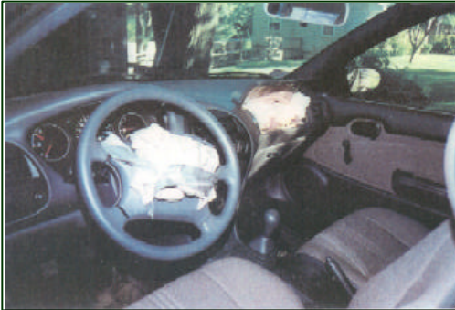
Figure 8. View of the deployed front left air bag and the deformation to the steering wheel rim.
