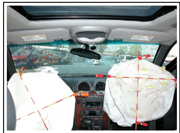
Figure 5. Deployed front air bags.
