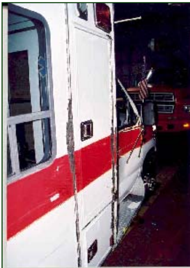
Figure 14. Asphalt embedded into the aft side of the door hinges.
