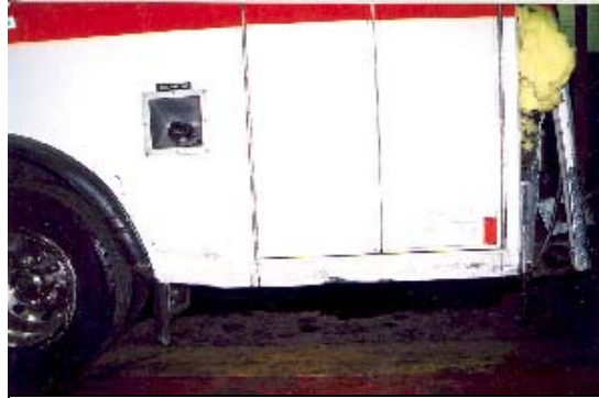
Figure 11. Left side damage from the initial impact with the taxicab.
