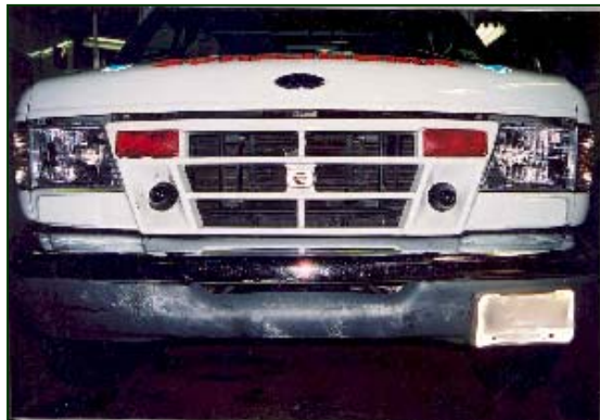
Figure 12. Frontal damage from the impact with the parked Dodge Caravan.
