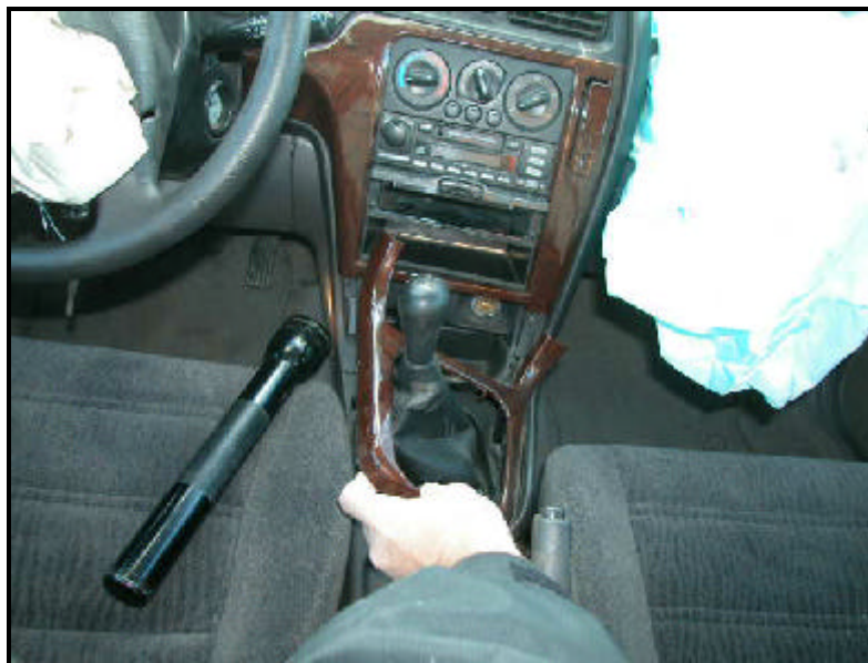
Figure 11. Displaced console trim
