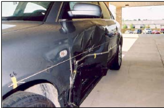
Figure 4. Damage to the left side of the Passat.
