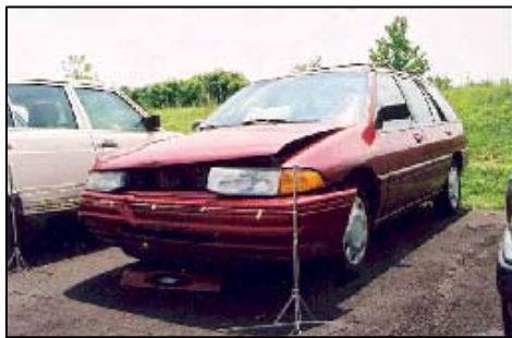
Figure 6. Frontal view of the Escort's damage.
