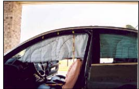
Figure 8. Deployed side impact air bag and side curtain.
