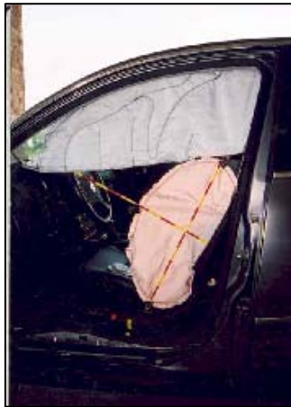
Figure 9. Exterior view of the deployed front left side air
