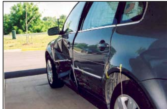
Figure 5. Continuation of damage on quarter panel.
