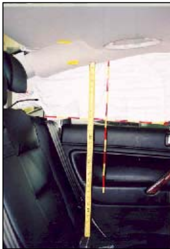
Figure 12. Vertical profile of the rear left side curtain.
