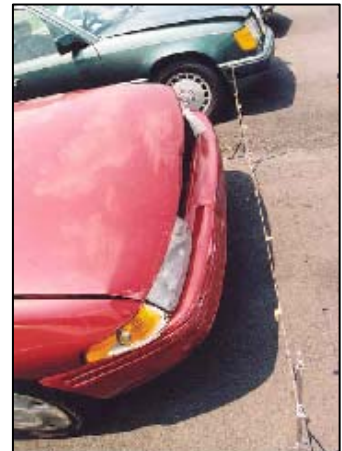
Figure 7. Right profile view of the frontal crush.
