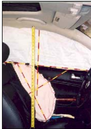
Figure 10. Interior view of the front left air bags.
