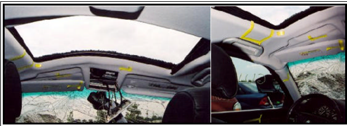
Figure 7. Contact evidence along the interior roof structure of the 2001 BMW 740iL 4-door sedan.
