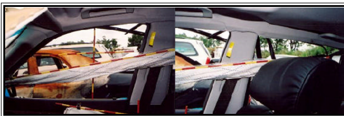
Figure 11. 2001 BMW 740il deployed right side head protection air bag.
