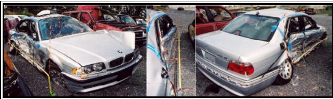
Figure 4. Right side surface damage to the 2001 BMW 740il 4-door sedan from the initial impact.
