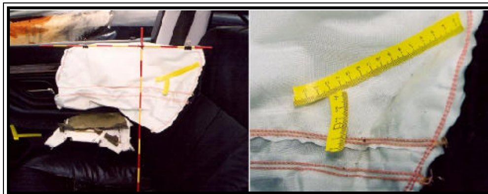
Figure 10. 2001 BMW 740il deployed right front side impact air bag (thorax).
