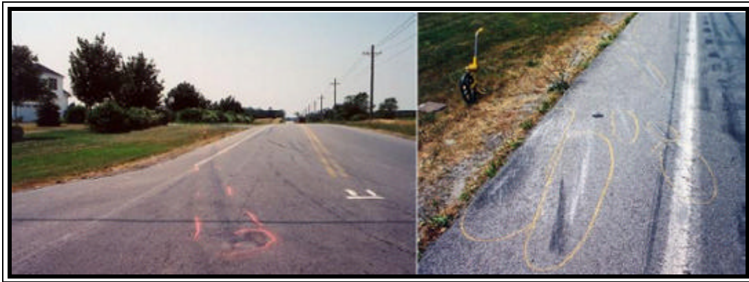
Figure 3. Southwest post-impact trajectory and pavement gouging for the 2001 BMW 740il.
