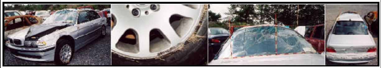
Figure 5. Rollover damage to the 2001 BMW 740il 4-door sedan.
