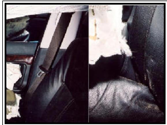
Figure 9. BMW front right restraint restricted in the stowed position by lateral component intrusions.
