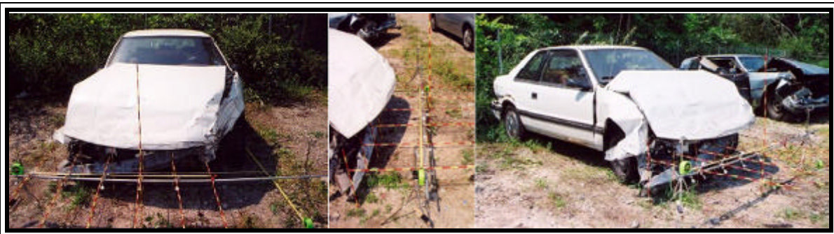
Figure 6. Frontal damage to the 1990 Dodge Shadow 2-door hatchback.
