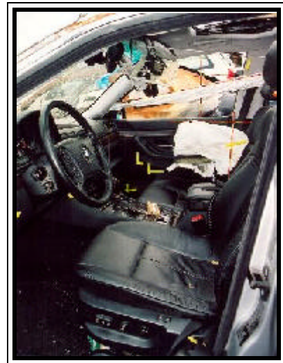
Figure 13. Lateral view of the 2001 BMW 740il front right passenger contact evidence.
