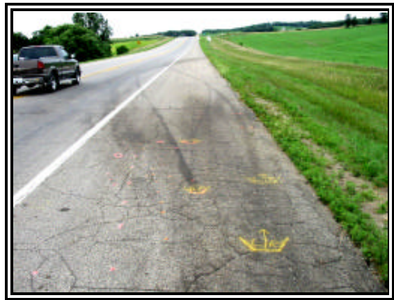
Figure 5. Post-impact skid marks from the Cavalier
