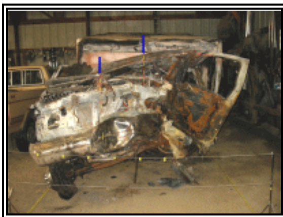
Figure 12. View showing the centerline variance between the windshield header and upper radiator support
