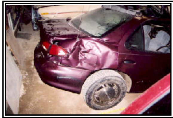
Figure 21: Side slap damage
