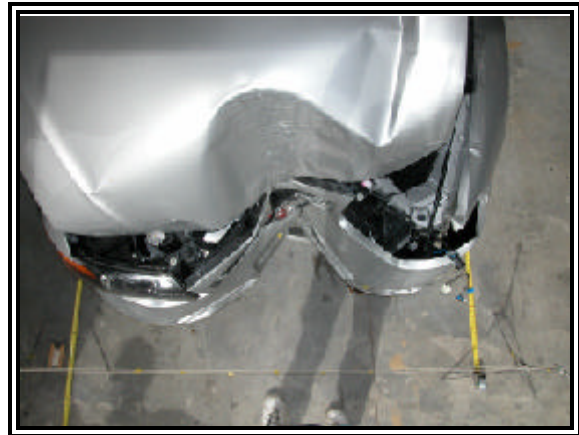
Figure 5: Overhead view of the frontal damage.
