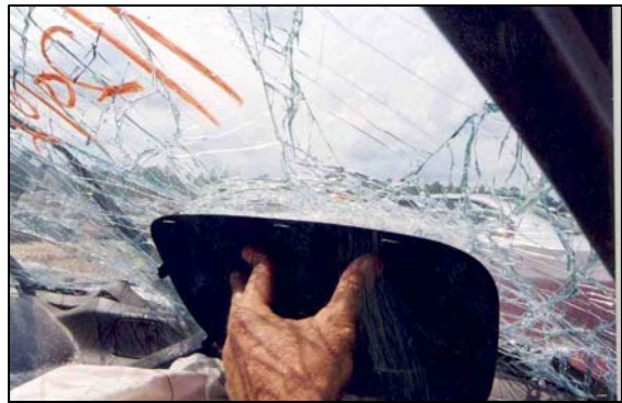
Figure 10 - Front right cover flap and windshield interaction.
