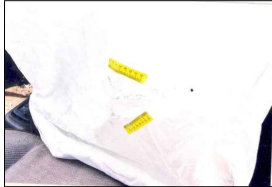
Figure 12 - Close-up of transfer evidence on front right air bag.
