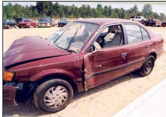
Figure 6 - Left side damage to the 1995 Toyota Tercel.
