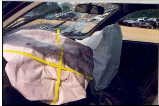
Figure 9 - View of driver's air bag.
