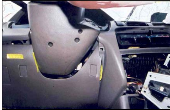
Figure 7 - Contact damage to knee bolster from driver's knees.
