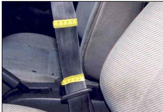
Figure 8 - Loading evidence on the driver's belt webbing.
