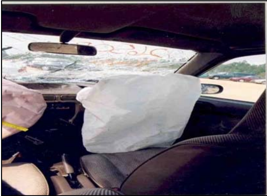
Figure 11 - View of the right front deployed air bag.
