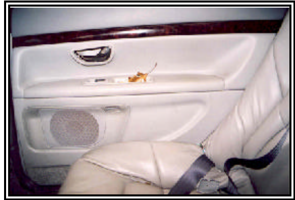
Figure 7: View of the rear right intrusion and seat compression.
