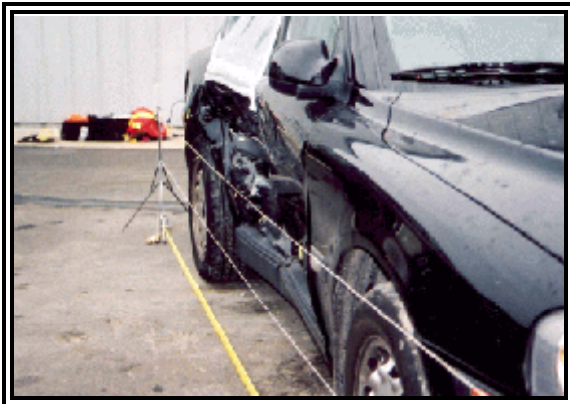
Figure 5: Right front close-up of the damage.
