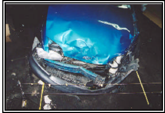
Figure 15: View of the frontal damage.
