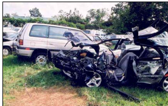
Figure 4 - Oblique view of damaged 2002 Ford Taurus SE.
