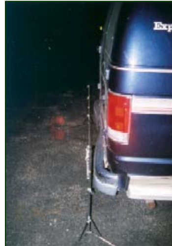
Figure 6. Extent of crush to the mid point of the rear bumper.
