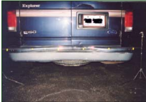
Figure 5. Rear bumper damage to the conversion van.
