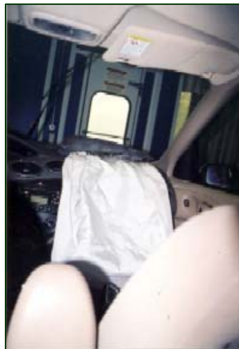
Figure 13. Deployed front right passenger air bag.
