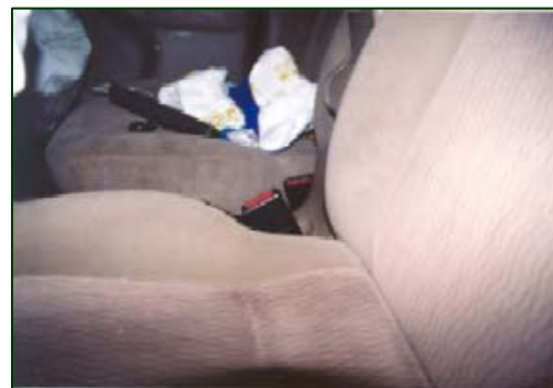
Figure 7. Fired front right buckle pretensioner.
