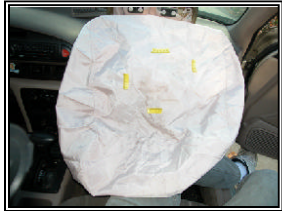
Figure 9: View of the PAB face.
