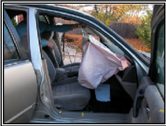
Figure 8: Right lateral view depicting the excursion of the air bag.
