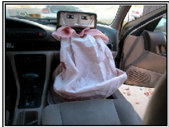
Figure 7: View of the deployed front right passenger air bag.
