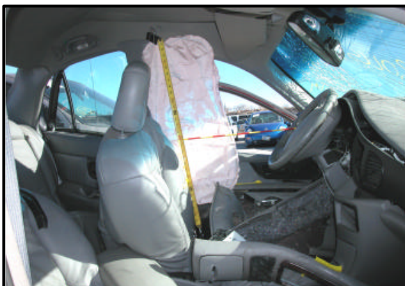
Figure 13: Right interior view of the SAB removed and unfolded from the module by the SCI investigator..
