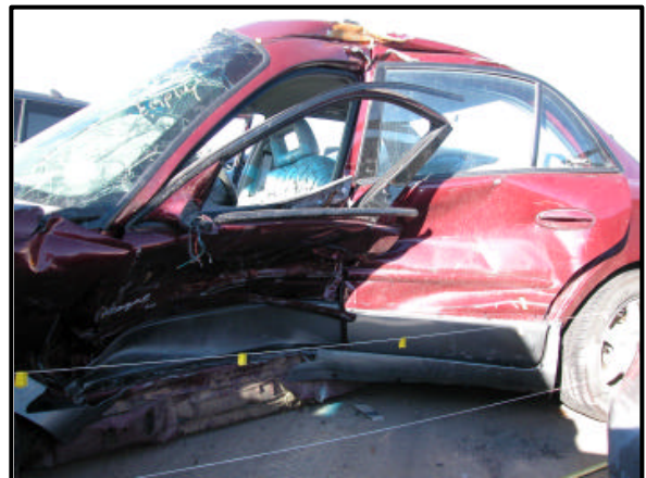
Figure 5: Close-up view of the left side damage.
