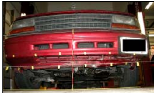
Figure 8. Frontal view of damage to bumper and lower radiator support
