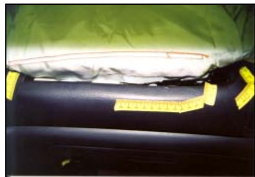
Figure 16. View of corner tears and faint transfer on the instrument panel adjacent to the leading edge of the cover flap
