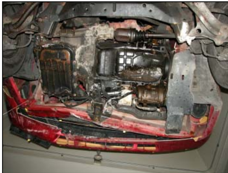
Figure 9. Undercarriage view showing damaged components and crushed lower radiator support
