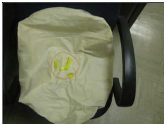
Figure 10. Removed driver's air bag. Occupant contact on center of air bag.
