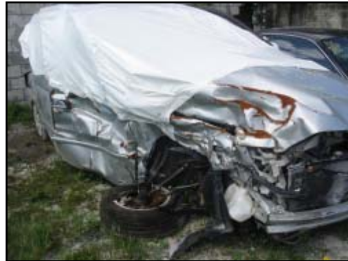
Figure 7. View of damage from the initial impact with the Jeep.
