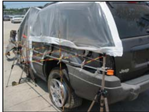
Figure 11. View of damage from second impact with the Honda.
