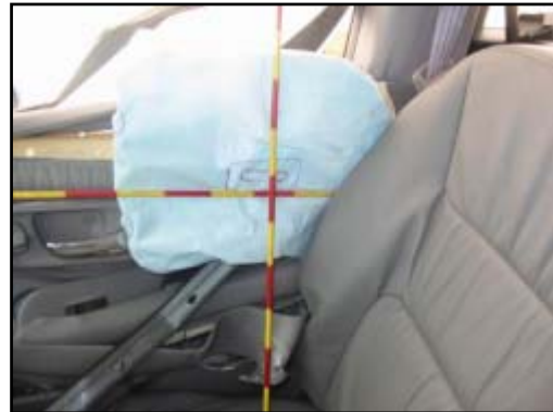
Figure 13. Deployed right side impact air bag.
