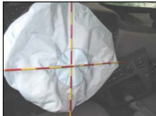
Figure 12. Deployed driver's frontal air bag.
