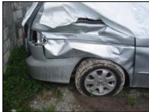
Figure 8. View of damage from second impact with the Jeep.
