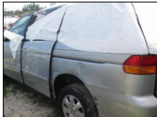
Figure 6. Sideswipe damage from impact with the Ford.
