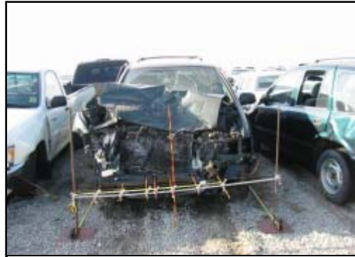
Figure 18. Damage sustained from frontal impact with the Chevrolet.
