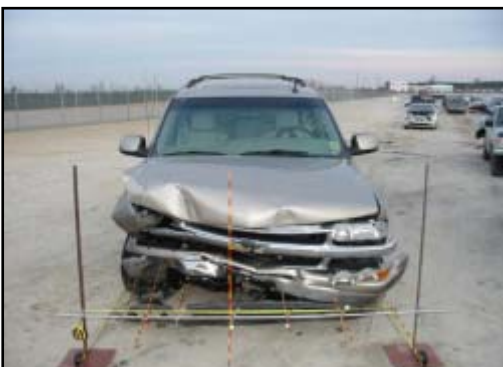
Figure 11. The damage from the signpost is located left of center.
