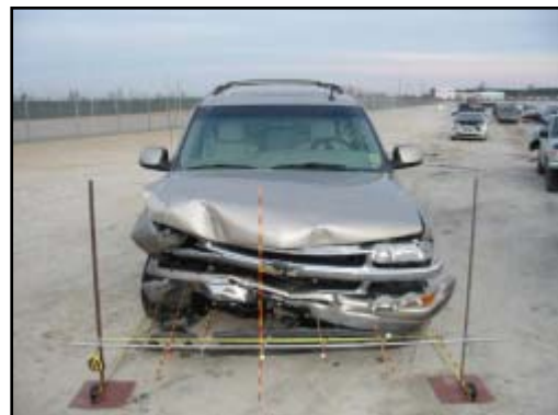
Figure 15. Damage from impact with the Toyota.
