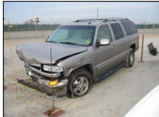
Figure 14. Area of damage from impact with the Geo.
