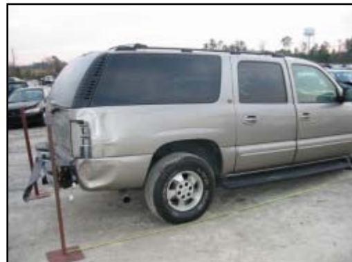
Figure 13. Area of damage from tree and signpost.
