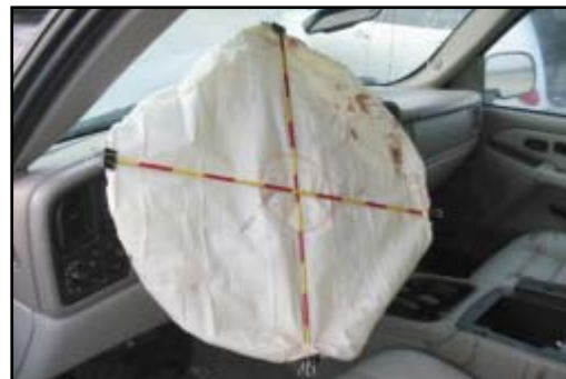
Figure 20. Deployed driver's frontal air bag. Note body fluid is a result of driver bleeding on the air bag and not from contact.
