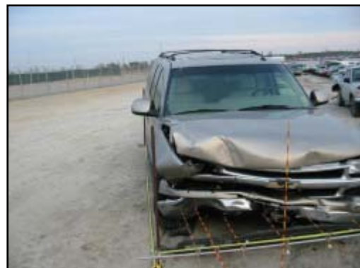
Figure 16. Damage from guy wire impacts is right of the center.
