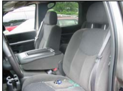
Figure 9. Integrated restraints in the Avalanche.
