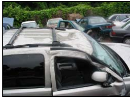
Figure 6. Roof and right side damage from rollover.
