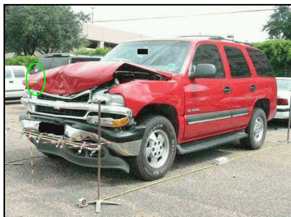
Figure 10: Other vehicle' s front and left side; highlighting shows where the case vehicle driver' s head left an imprint
