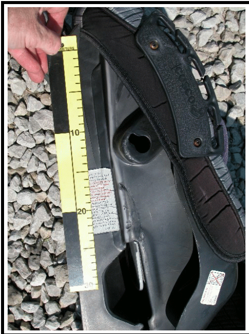
Figure 15. Side view of CSS showing seat back fracture
