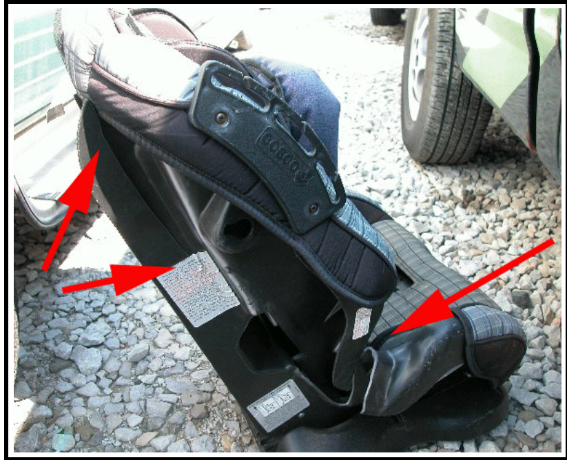
Figure 14. Shell fractures to seat back and side panel
