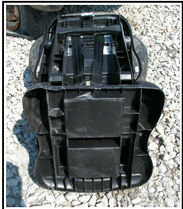
Figure 16. Bottom of child seat—shows compression to left side of base.
