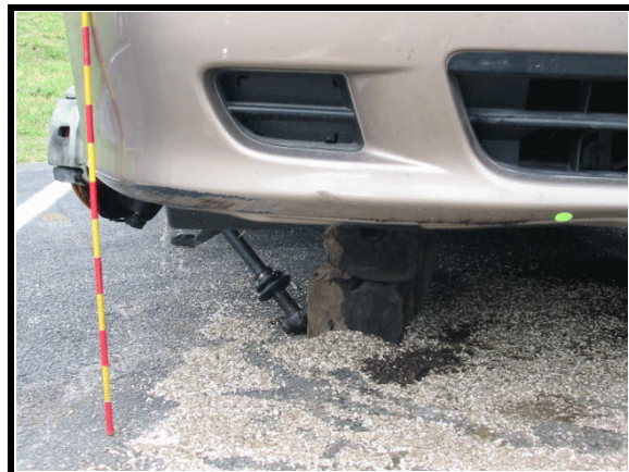
Figure 6. Close up of damage to front right bumper fascia
