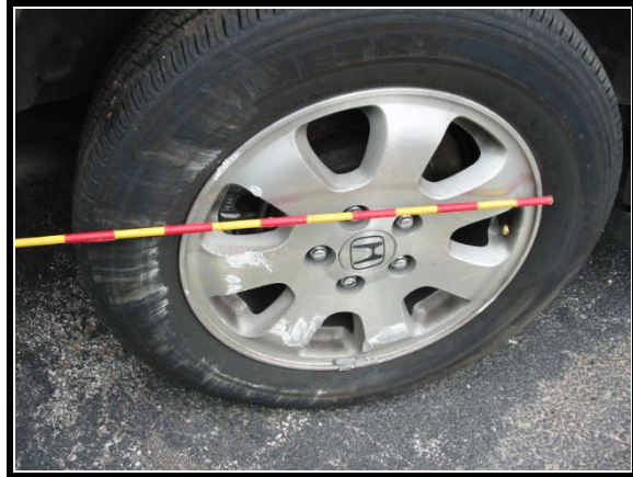
Figure 7. Damage to right rear wheel
