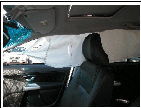
Figure 13. Interior view, right side air curtain
